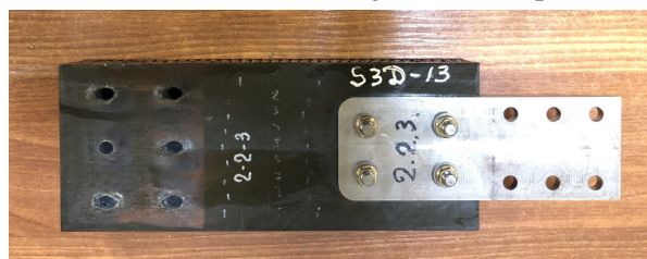
Fig. 5. Service hole elongation after the end of fatigue test
